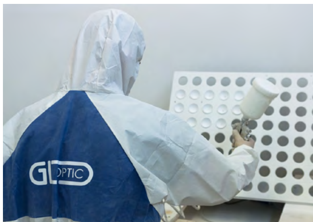
Fig. 6. Painting of integrating spheres with barium sulphate.
