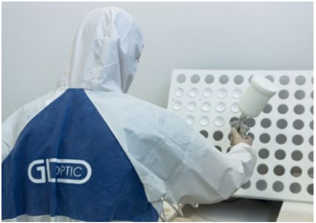
Fig. 6. Painting of integrating spheres with barium sulphate.
