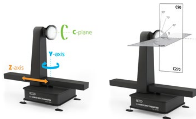
Fig. 3. Type C goniometer with three mechanized axes and schematic diagram of creating goniometric files for a typical luminaire.
